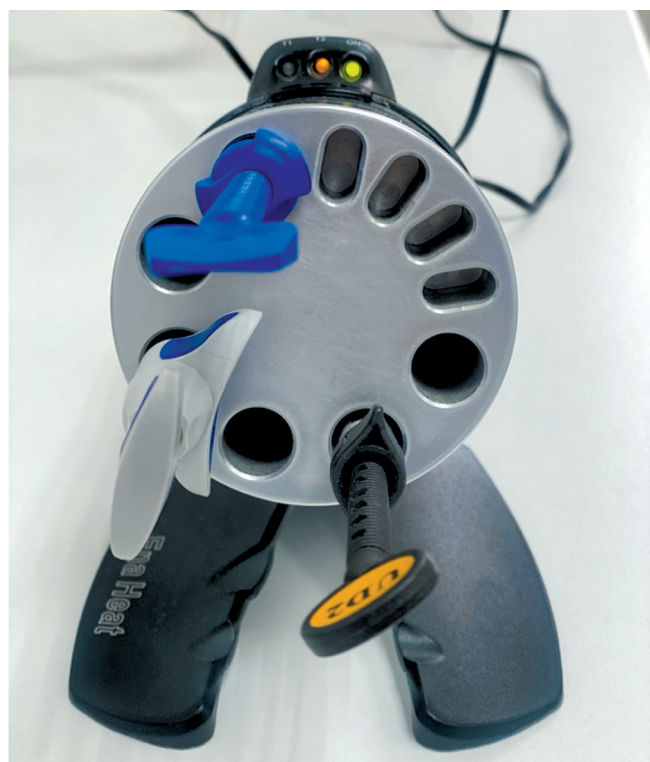
Fig. 2. Furnace (Micerium; Avegno, Italy) for heating composite materials. T2- mode 55°C.
