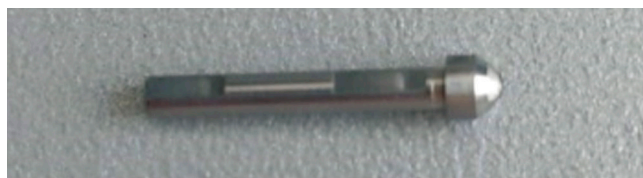
Fig. 4. Berkovich indenter (a truncated three-sided diamond pyramid) with a device for measuring microhardness
