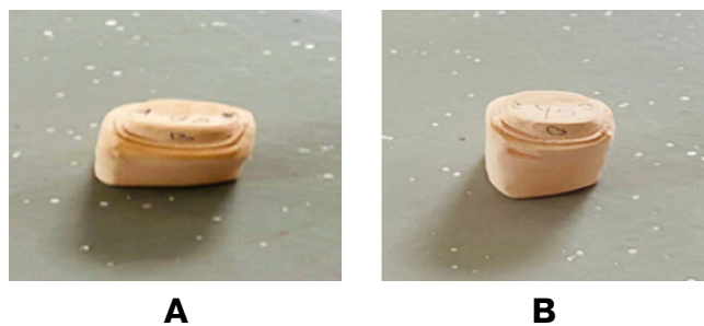
Fig. 1. Master die with a different finishing line: A – 90° shoulder and B – 45° chamfer
