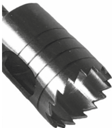
Fig. 2. Working part of device (trepan) with triangular cutting teeth
