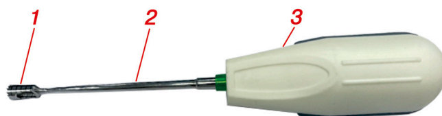
Fig. 1. Device for manual unstressed mucotome-osteotome for taking a three-layer autograft from the tubercle of the upper jaw: 1 – working part (trepan); 2 – rod; 3 – handle
