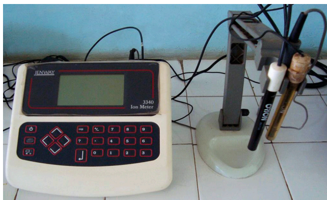
Fig. 2. Fluoride Electrode with Ion Analyser
